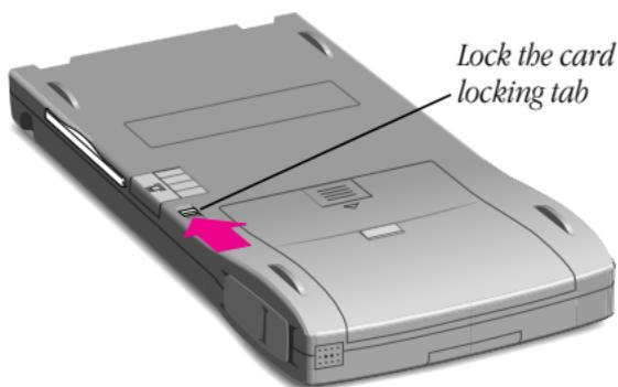
When you insert the card, make sure you push it all the way into its slot and lock the locking tab. When you lock the locking tab, your MessagePad takes a few moments to examine the card. When your MessagePad is ready to use the card, a slip appears with information about the card.
