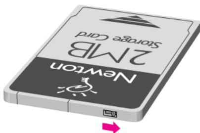
To unlock the card, slide the write protection switch back toward the center of the card.
