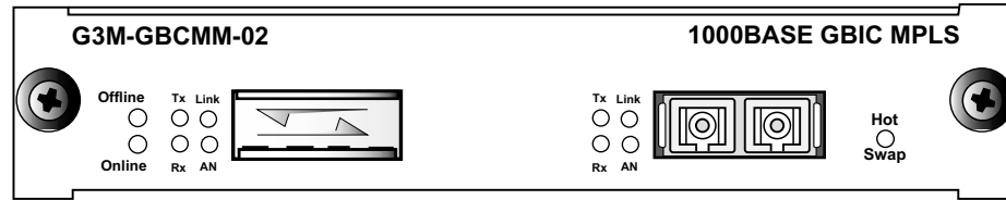
Figure 2-8 Front panel of MPLS GBIC line card with one GBIC installed
