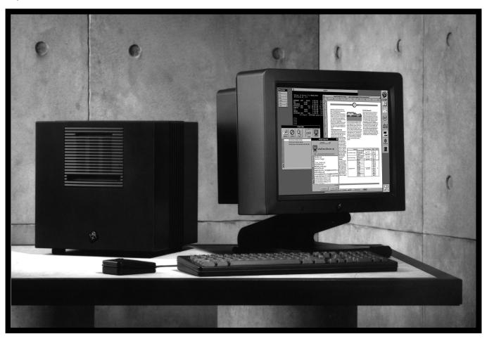
The NeXTcube is a versatile, easy-to-use workstation that can be utilized as a desktop monochrome system, true color 32-bit-per-pixel color/video workstation or file server system, all featuring NeXT's object-oriented operating and development environment.
