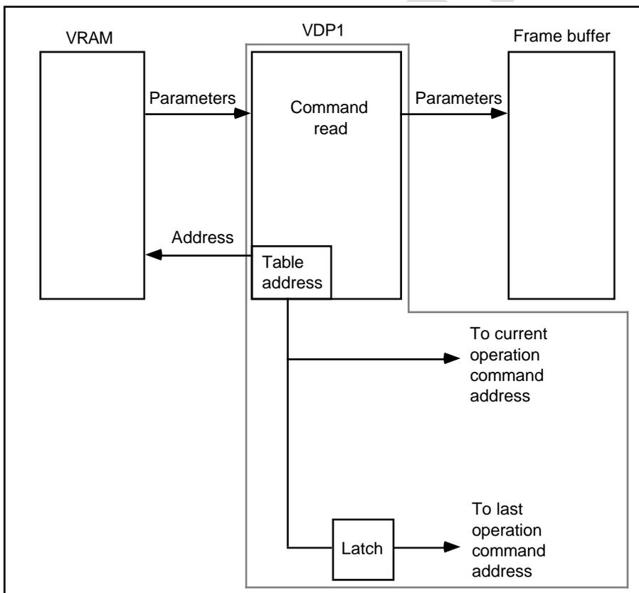
Figure 4.3 Last Operation Command and Current Operation Command Address
