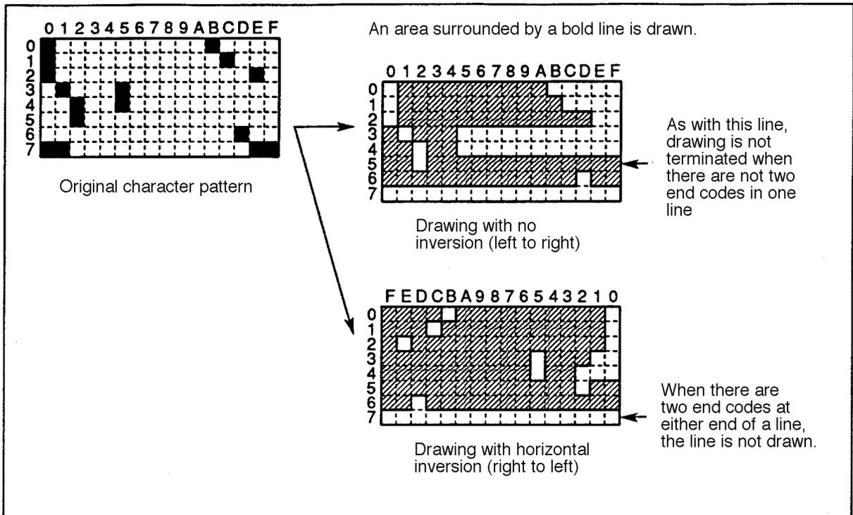
Figure 6.10(a) End Code Processing (1 of 2)
