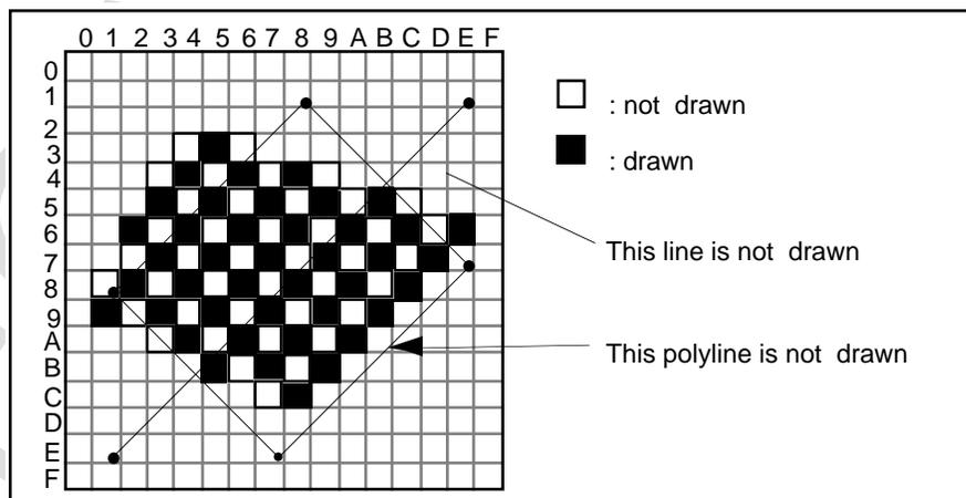
Figure 6.9 Mesh Processing of Lines and Polylines
