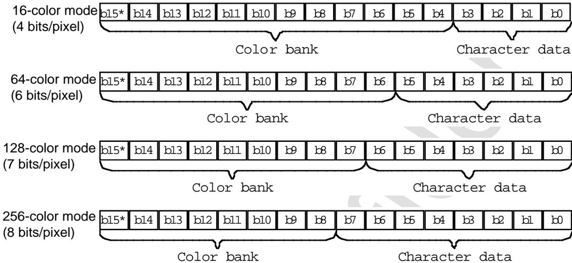
Note: b15 = 0 when RGB data are mixed; b15 can be either when not mixed.
