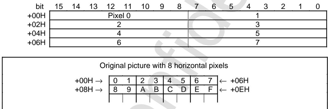
Figure 6.12 Example of Drawing in Modes 2, 3, and 4
