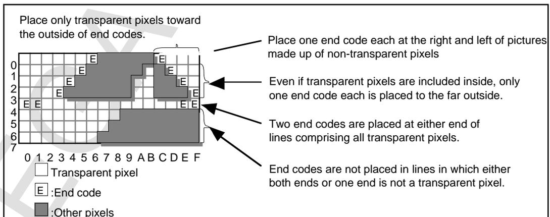
Figure 6.10(b) End Code Processing (2 of 2)
