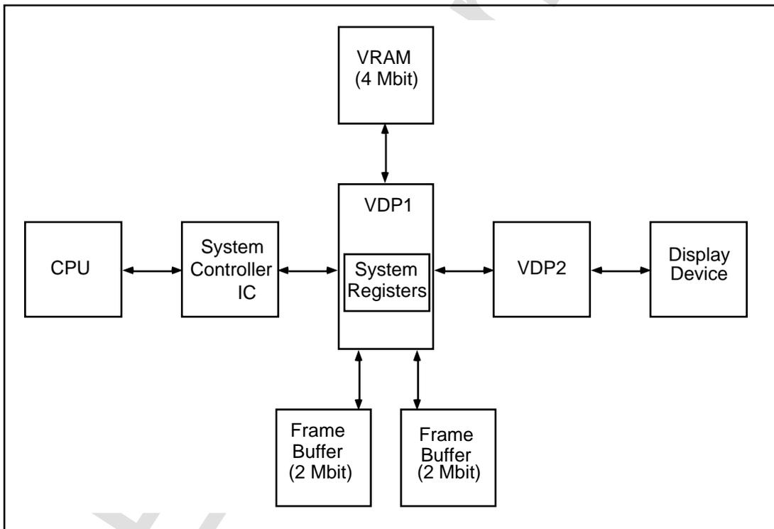
Figure 1.1 System Configuration
