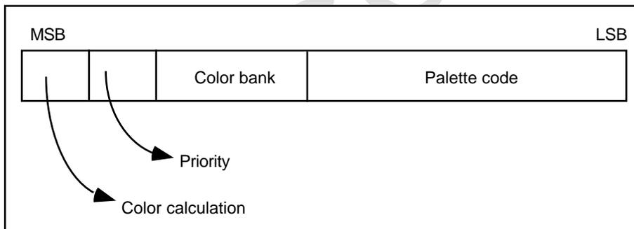
**Figure 1.10 Bit Configuration of Color Bank Method**
