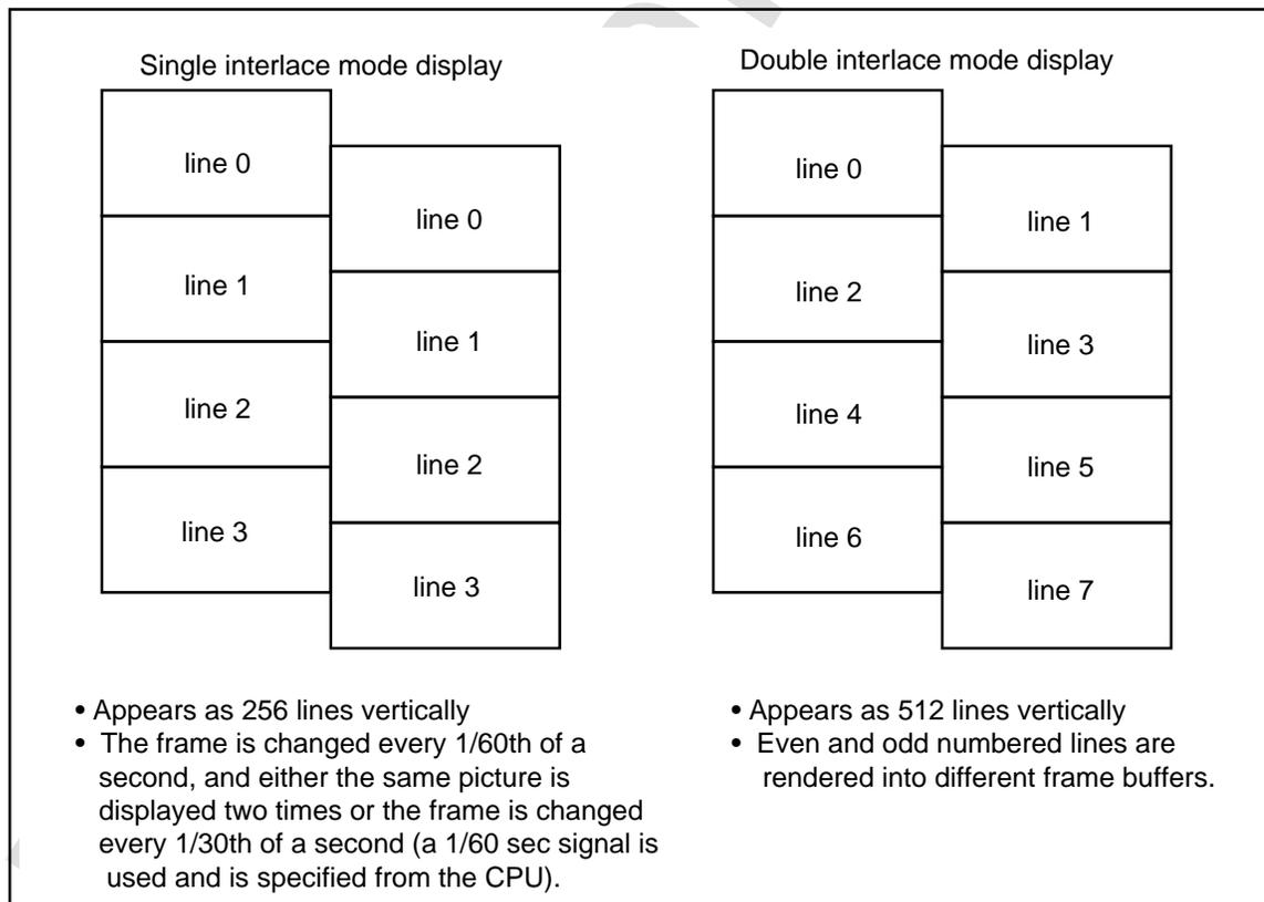
**Figure 4.1 Single Interlace and Double Interlace Display**
