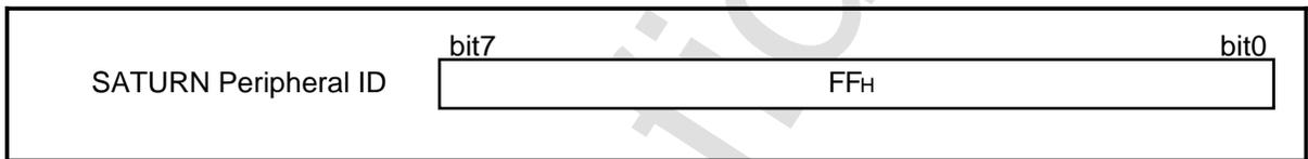
**Figure 3.19 SATURN Peripheral ID when Tap Unconnected**
