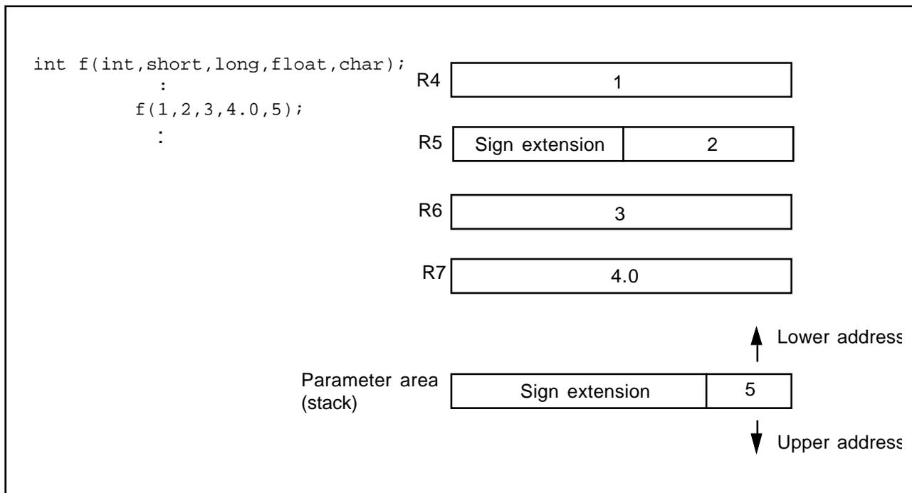
**Example 3:** Parameters having a type that cannot be allocated to registers from R4 to R7 are allocated to the stack area.
