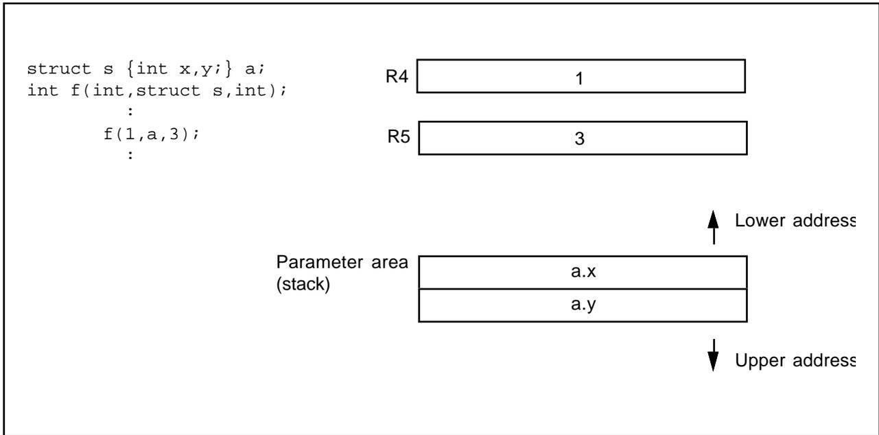
**Example 4:** If a function whose number of parameters changes is specified by prototype declaration, parameters which do not have a corresponding type in the declaration and the immediately preceding paramters are allocated to a stack.
