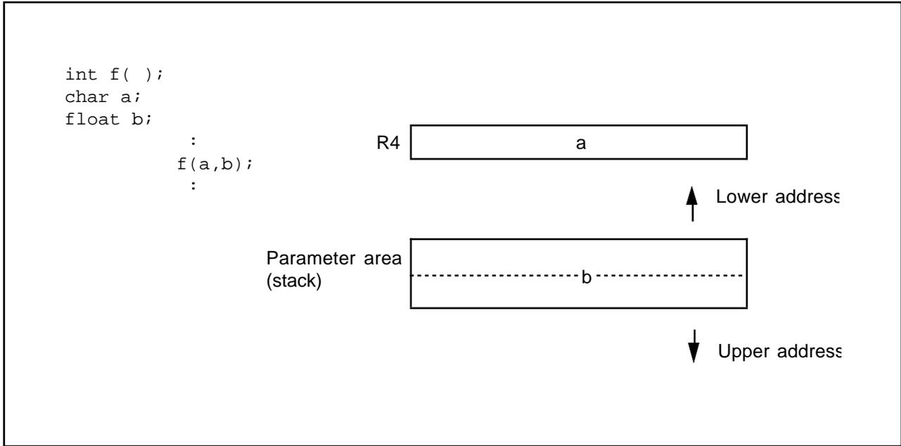
**Example 6:** If a value returned by a function exceeds 4 bytes, or is a structure type, a return value is specified just before parameter area. If structure size is not a multiple of four, an unused area is generated.
