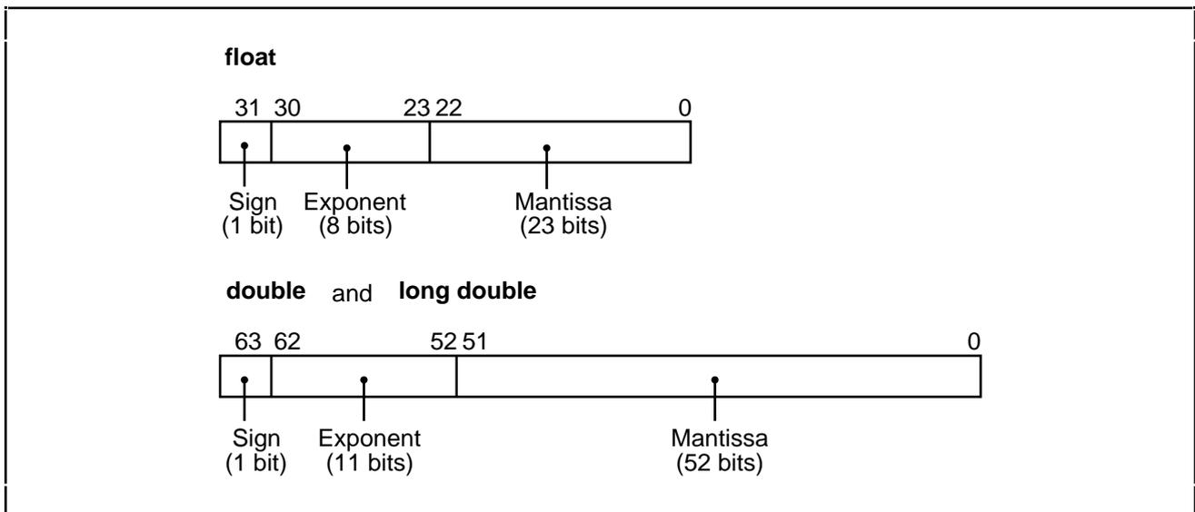
**Figure A-1 Structure for the Internal Representation of Floating-Point Numbers**
