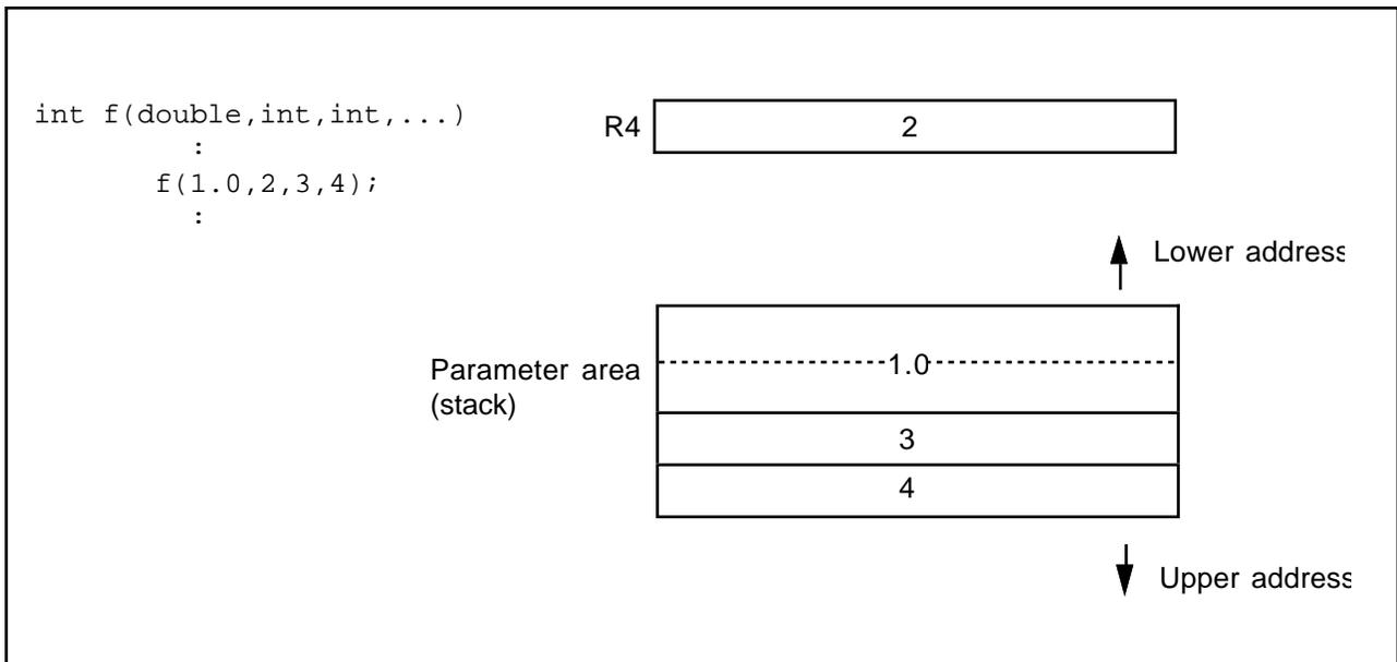
**Example 5:** If no prototype is declared, **char** and **float** types are extended to **int** and **double** types, respectively.
