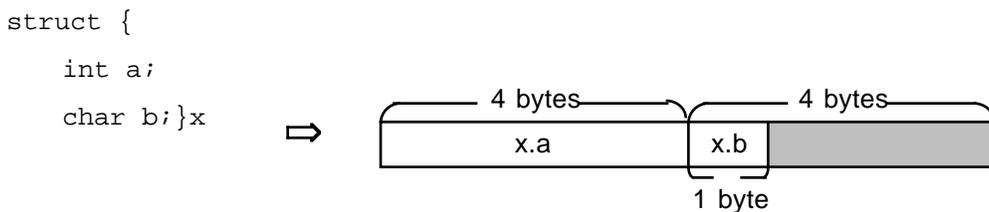
\*2. When an union has 4-byte alignment and the maximum size of its members is not a multiple of four, the remaining bytes up to a multiple of four are included in this union.
