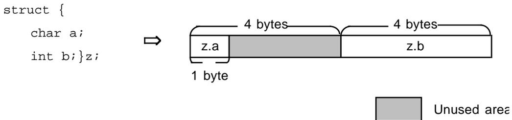
If a structure has 4-byte alignment and the last member ends at an address indivisible by four, the remaining bytes are included in this structure.
