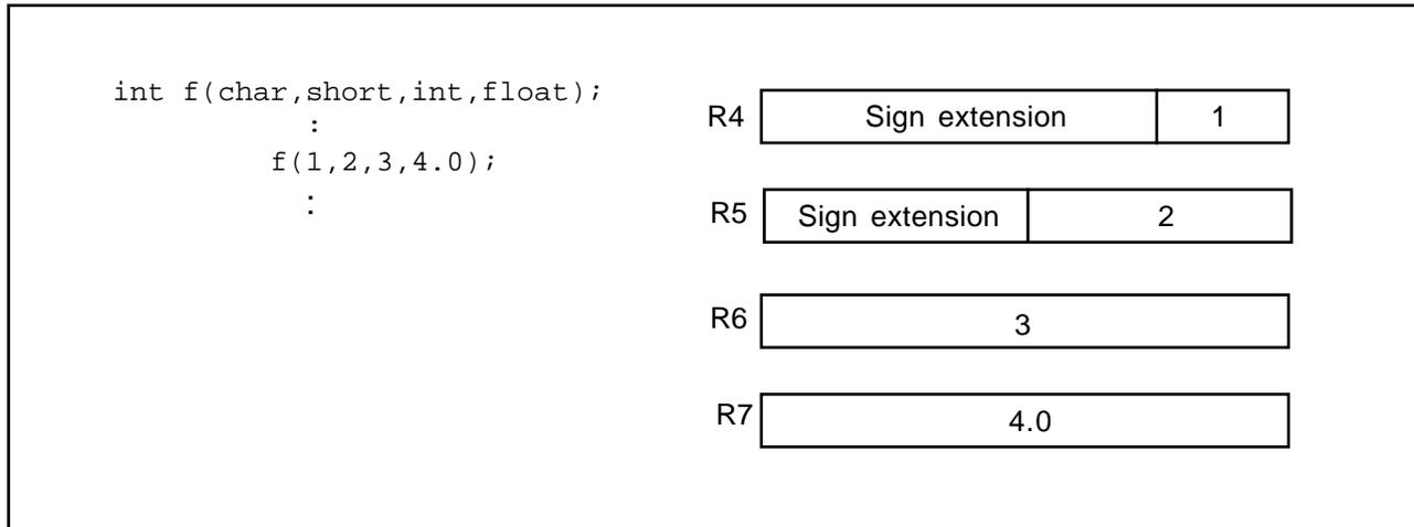
**Example 2:** Parameters which could not be allocated to registers from R4 to R7 are allocated to the stack area as shown below. If a **char (unsigned)** or **short (unsigned)** type parameter is allocated to a parameter area on a stack, it is extended to a 4-byte area.
