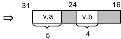
z If an anonymous bit field member or a bit field member with a bit field size of 0 is declared, the next member is allocated to the next area.
