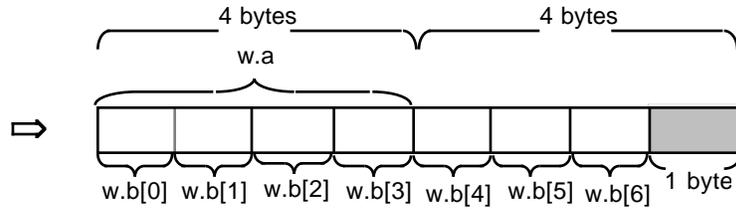
**Bit Fields:** A bit field is a member of a structure. This part explains how bit fields are allocated.
