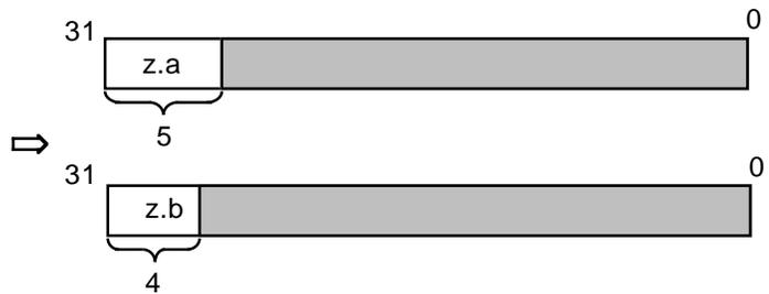
y If the number of remaining bits in the area is less than the next bit field size, though type specifiers indicate the same size, the remaining area is not used and the next bit field is allocated to the next area.
