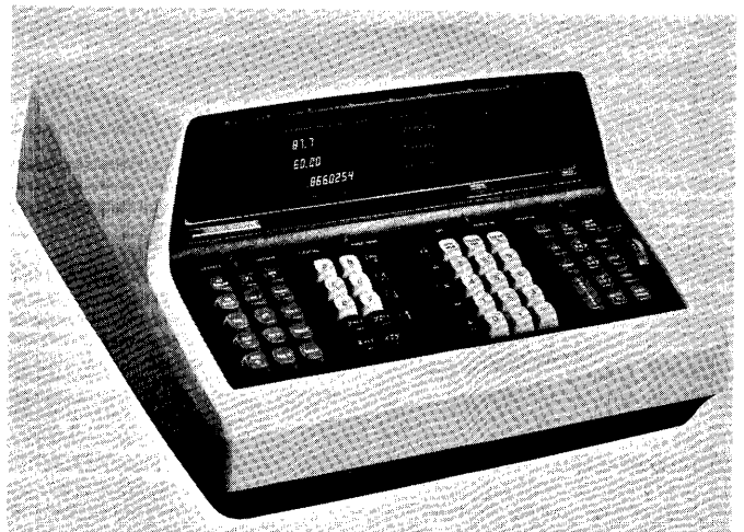
Fig. 1. This new HP Model 9100A calculator is self-contained and is capable of performing functions previously possible only with larger computers.
