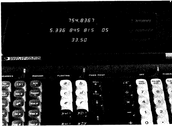
Fig. 2. Display in fixed point with the decimal wheel set at 5. The Y register has reverted to floating point because the number is too large to be properly displayed unless the digits called for by the DECIMAL-DIGITS setting are reduced.
